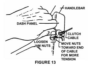
**3.5.1 TENSION TEST:** Start the engine with tiller in neutral. Shift transmission into FWD & TILL and pull the wheel and tine control bail up against the handle bar. Tines and wheels will start to rotate. Release control bail. Tines and wheels should stop rotating immediately. If rotation continues after release of control bail then clutch spring tension is to great and will have to be readjusted as described in BELT TENSION ADJUSTMENT Section.
